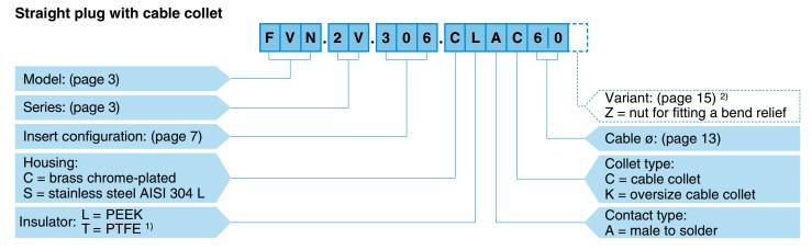
**FVN.2V.306.CLAC60** = straight plug with cable collet, 2V series, multipole type with 6 contacts, outer shell in chrome-plated brass, PEEK insulator, male solder contacts, C type collet for 6 mm diameter cable.
