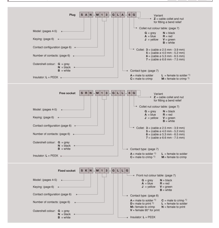
**SAN.M13.GLA.6G** Straight plug with cable collet and alignment key (N), multipole type with 13 male contacts to solder, grey Proprietary sulfone shell, PEEK insulator, collet for max cable ø 6.5 mm and grey collet nut.
