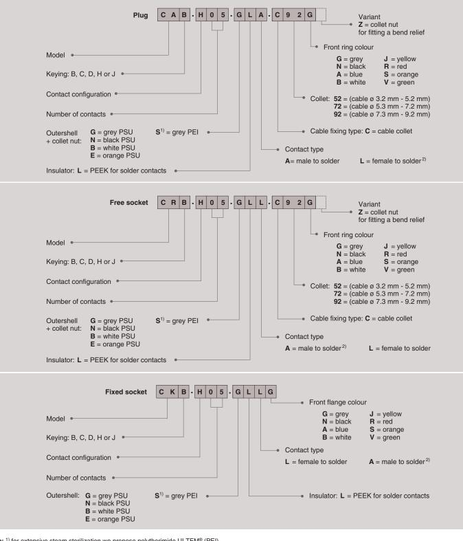
Note: <sup>1)</sup> for extensive steam sterilization we propose polytherimide ULTEM<sup>®</sup> (PEI). <sup>2)</sup> model available only with H and J keying (inverted contacts).
