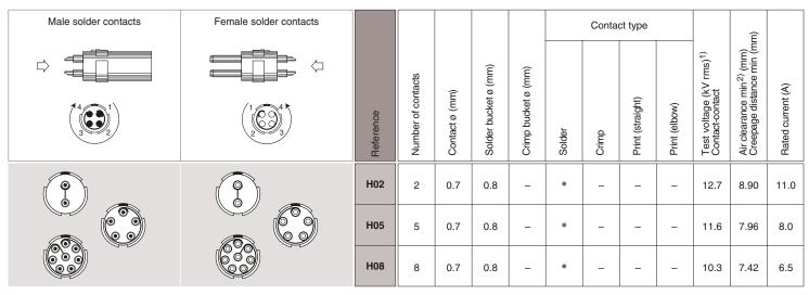
Note: 1) The use of potting type Epoxy\* (insert config. H02, H05 and H08) or adhesive-lined heatshrink tubes over each termination (only H02 and H05) is necessary to guarantee the indicated Test voltage.
