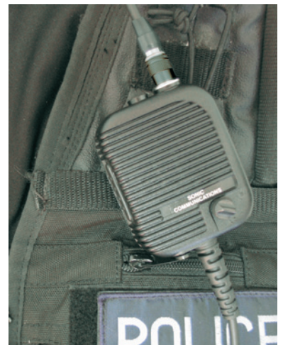
Firearms Remote Audio Terminal with K series connectors. (Sonic Communications Ltd, UK)
