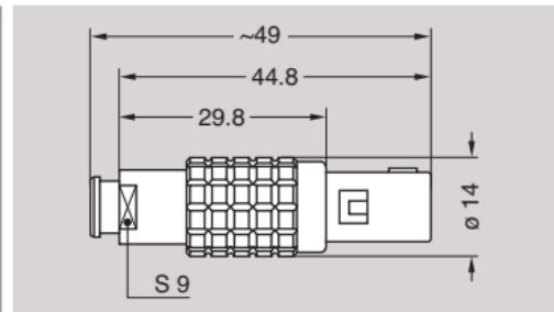
**Note:** Replace ●.● by contact configuration. All dimensions are in millimeters.
