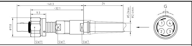
Outer shell Coupling nut Retaining ring Collet nut
