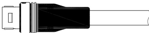
4. Slide the heat shrink tubing . With a heat gun fully shrink the tubing until it retracts .
