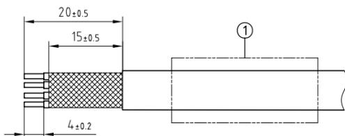
1. Strip the cable according to the given dimensions . Slide it into the heat shrink tubing ① ( not furnished ) .
