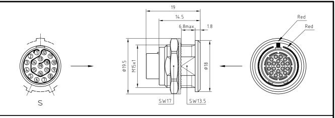
Outer shell Earthing crown Insulator Male contact
