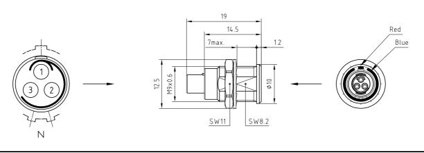
Outer shell Earthing crown Insulator Female contact
